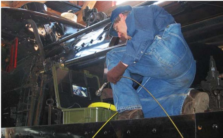
AoSRH chief mechanical officer, Tim Sposato, uses fiber-optic cable to inspect the flues, tubes and other internal components inside the boiler of ex-Canadian Pacific 4-6-2 No.1293 during this locomotive's annual inspection. As usual, No.1293 was found to be in perfect condition.
