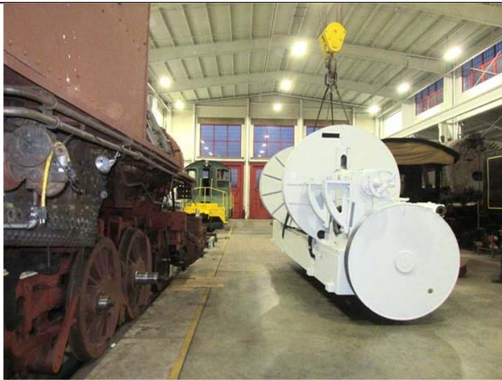
**The Putnam wheel lathe is moved into position by our back shop's 30-ton overhead crane.**
