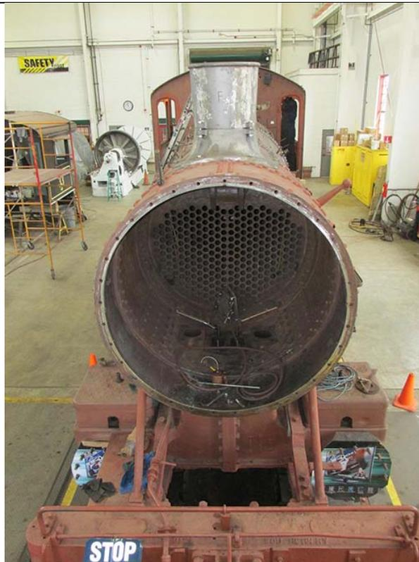
**No.12 Morehead & North Fork 0-6-0 showing new smokebox steel and new stack castings**
