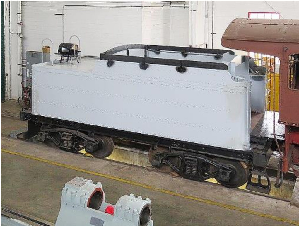
A brand-new fabricated tender tank on #12's rebuilt frame and trucks
