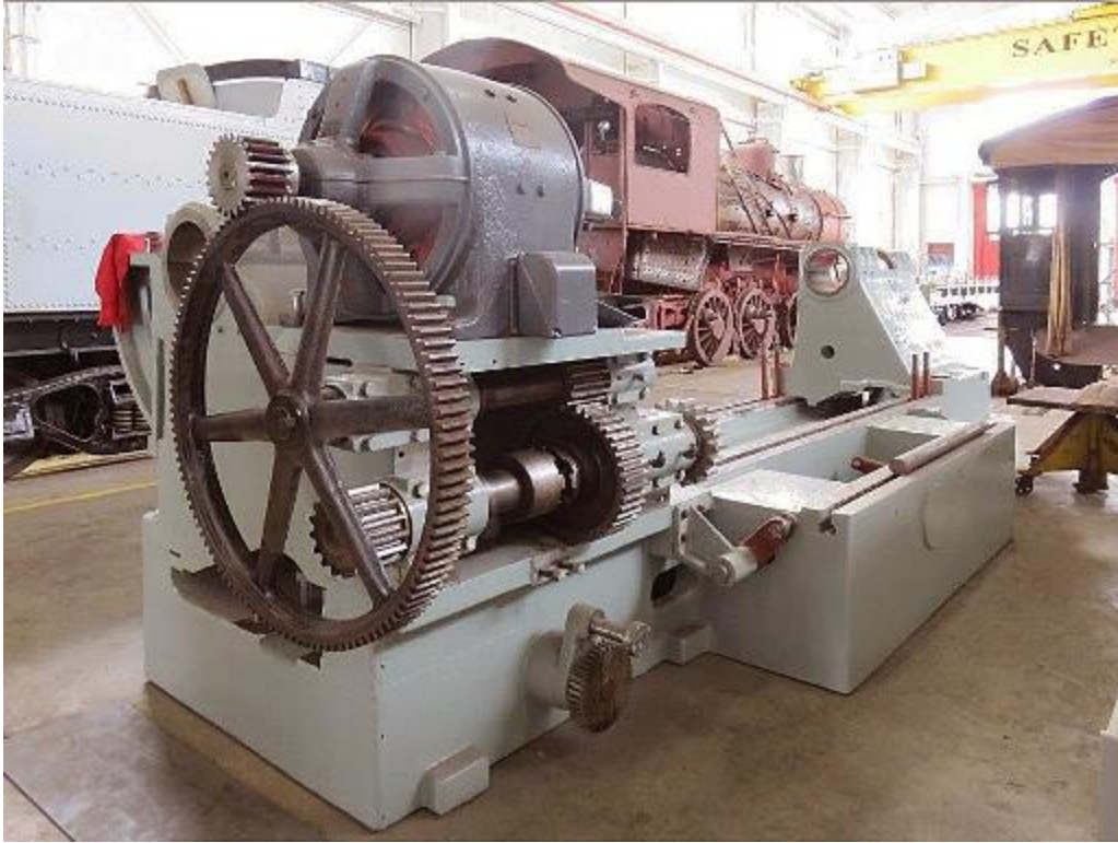
Putnam 80-inch wheel lathe under re-assembly
