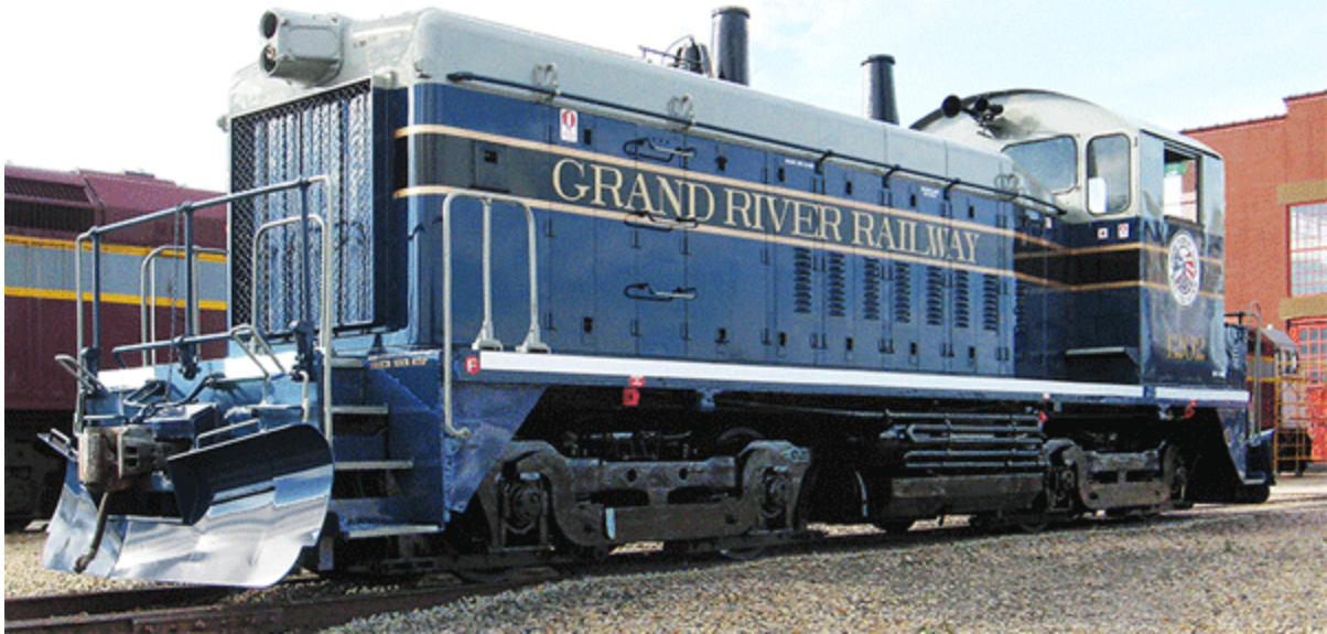
Former A&S SW1200 #1202 repainted in B&O inspired livery and fitted with snow plows for lease to Grand River Railway
