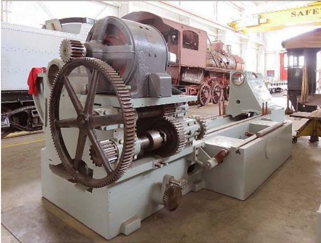
Putnam 80-inch wheel lathe under re-assembly
