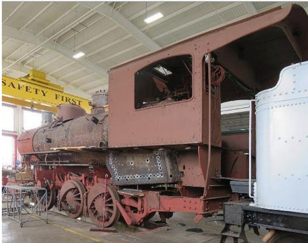
Former M&NF 0-6-0 #12 undergoing restoration
