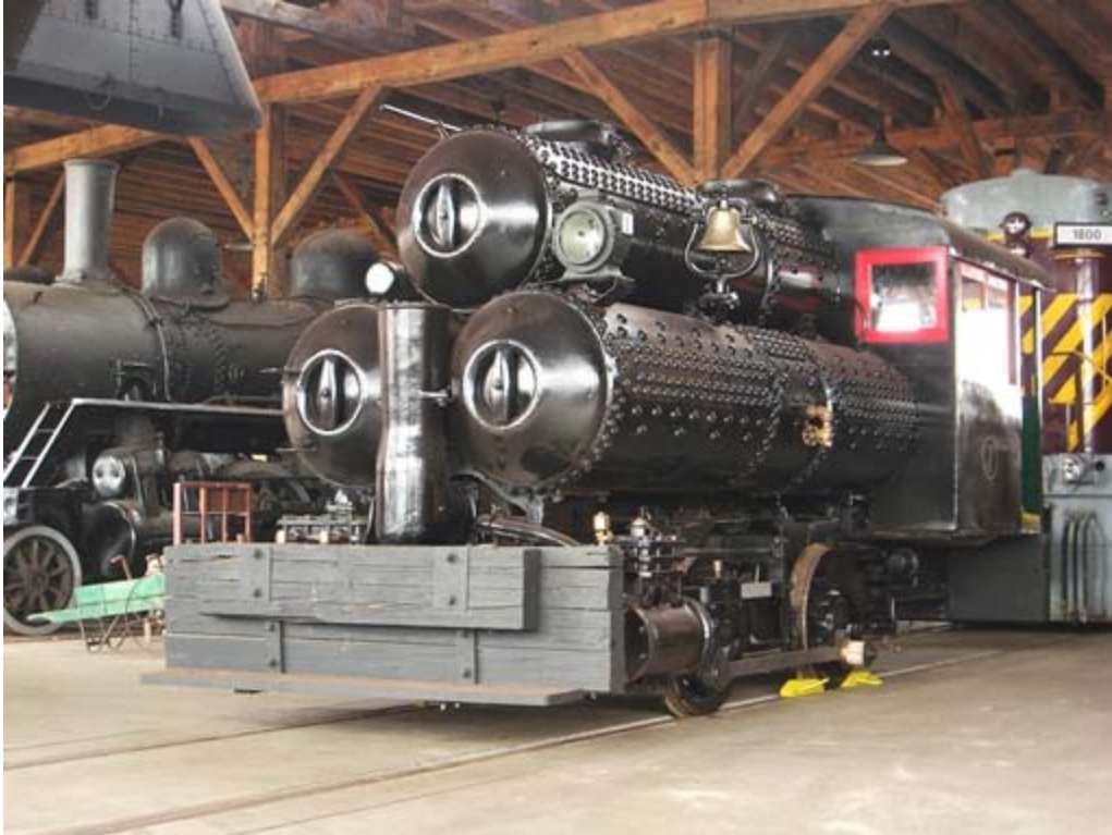
Compressed air locomotive #1 after cosmetic upgrades
